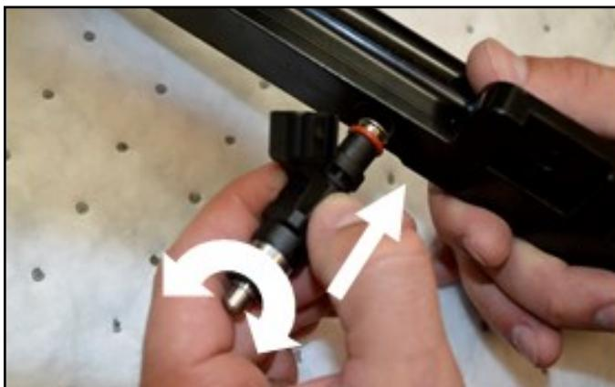
Apply a thin coat of engine oil to bottom o-ring on fuel injectors.
