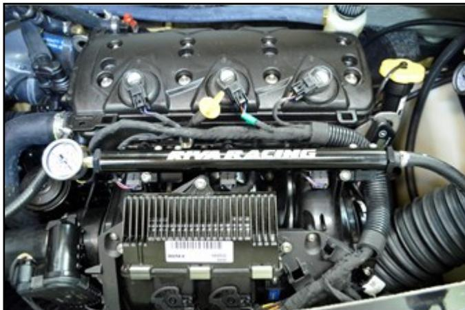
\* Shown in test configuration (with fuel pressure gauge). Remove gauge before riding or racing.
